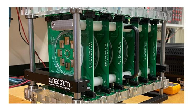
In this project, the effects of cosmic ray irradiation on the reliability of nano-scale gate-oxide layers are assessed under realistic electrical conditions. In a specifically developed test setup, power semiconductors provided by SwissSEM are exposed to proton and neutron irradiation while a gate voltage is being applied. The aim is to understand device failures related to cosmic ray irradiation into their gate oxide layers. The results of the project will support the
