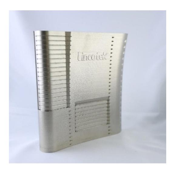
The applied material analytics of ANAXAM using Neutron Diffraction helps Lincotek Additive to analyze the residual stresses of Nickel based superalloys after the printing process and after additional post-SLM heat treatments. Since the SLM printing process is directional and the cooling rates during the printing process are very high, residual stresses in the printed parts
