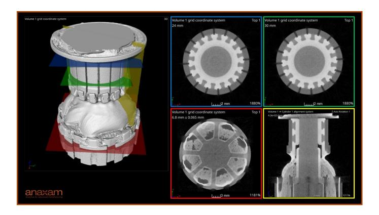
ANAXAM's material analytics - based on the most advanced possibilities in the field of measuring methods - using high-resolution Neutron CT was successfully applied to non-destructively and three-dimensionally characterize electric motors of hot air blowers. The analysis results support Leister in achieving
